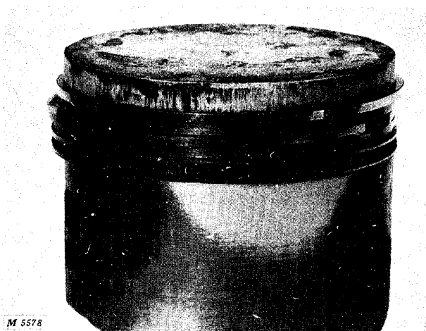
Fig. 9-Scored Piston and Rings
