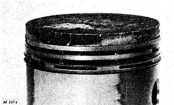
Fig. 19-Piston Top Land Burning Caused by Detonation
