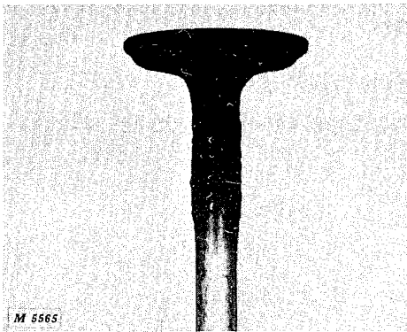
Fig. 5-Gummy Valve Causing Valve to Stick
