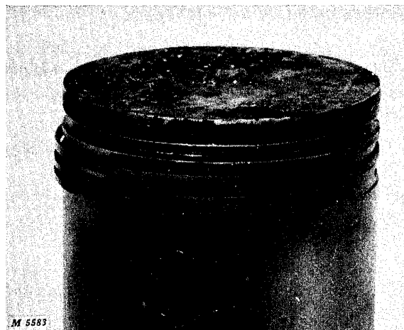
Fig. 14-Worn Oil Rings Which Cannot Provide Oil Control
