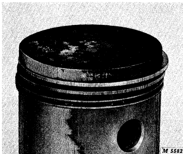
Fig. 13-Scratched Ring Faces Caused by Abrasives in the Engine
